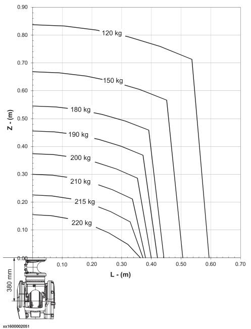
1.5.3 Maximum load and moment of inertia for full and limited axis 5 (center line down) movement
