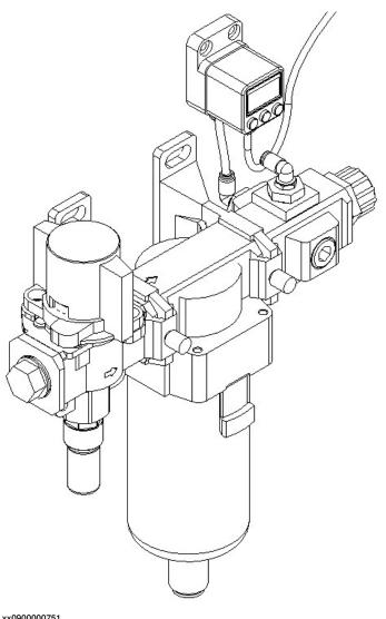
The air supply circuit ends with a Swivel Nut adapter (suitable for a Swivel Nut adapter 20 078 A, we recommend a Parker 39C82-15-8BK fitting).
